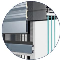
SKB Styroterm has been designed to be completely installed into the insulation so that the box becomes an unnoticeable element of the façade.
