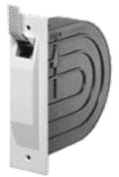
For manual control of top-mounted (version with a wound up tape) and adaptation roller shutters (version without a tape in the winder), max load capacity is 11 kg. Can be mounted in the wall as well as in the window frame.
